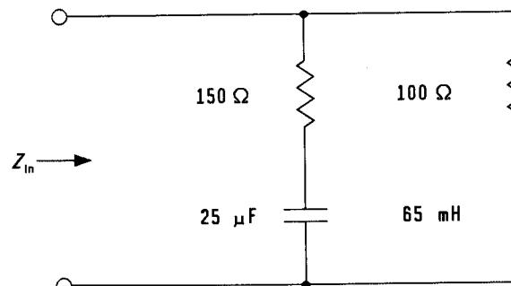
The elements in series are simply added to give the branch impedances  $Z_1 = 150 - i106.1033$  and  $Z_2 = 100 + i24.5044$ . The circuit is redrawn below.
