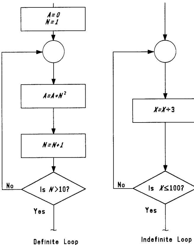
The definite loop illustrated in the figure will generate the sum of the squares of the integers 1 through 10. Notice that  $A$  is 0 initially, the loop counter  $N$  is 1 initially, and the loop counter is incremented by 1 with each pass through the loop. The definite loop is performed a *fixed* number of times (10 in this case). On the other hand, the indefinite loop repeats *indefinitely* until the desired condition ( $X \leq 100$ ) is met.
