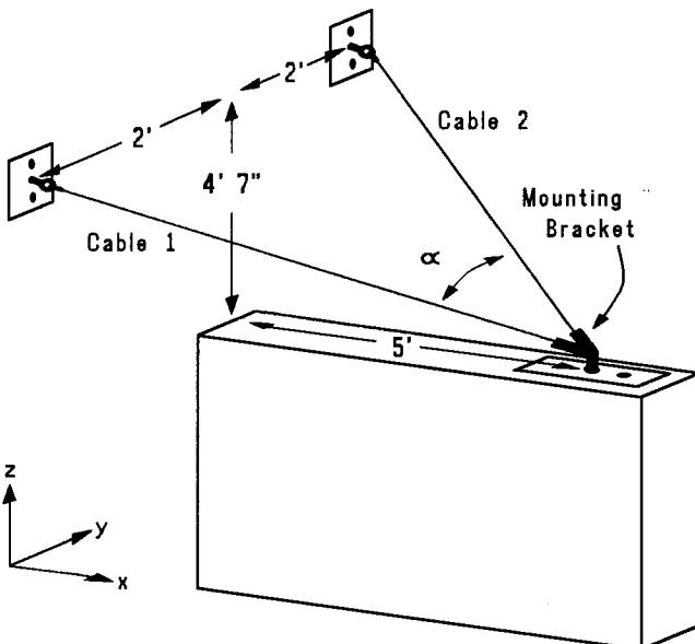
Represent the cables as vectors going *from* the wall *to* the brackets and compute the angle  $\alpha$  between them for the bracket angle. For the length of cable needed, find the magnitude of the vector representing one cable. By symmetry, the total cable length is twice this.
