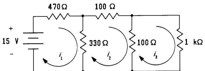
The following 3 equations are generated by summing the voltage drops around each loop.
