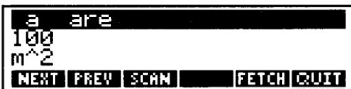
The top line shows the unit abbreviation of the selected unit, in this example **a**, followed by the full name, **are**. **Are** is the first unit in the HP-28C alphabetical unit catalog. The second line shows the unit's value in SI base units, which are shown in the third line. Altogether, this display shows that **are** is abbreviated **a** and has the value 100 meters squared.
