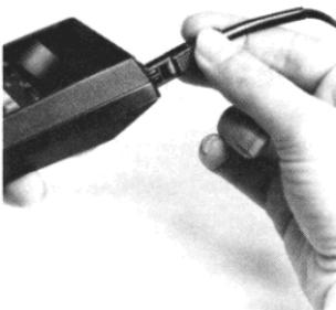
2. Press down on the short ridges of the battery door, close to the edge, until the door release snaps open. Slide the door open.
