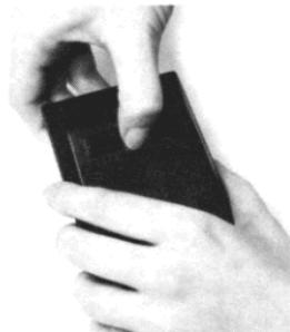
3. When door is removed, turn calculator over and gently shake, allowing the battery pack to fall into the palm of your hand.
