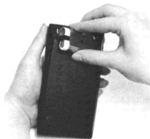
5. Insert battery door and slide door back into place.
