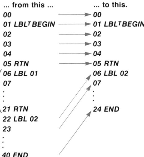
With the calculator set to line 6, **DEL** 016 would delete 16 lines.
