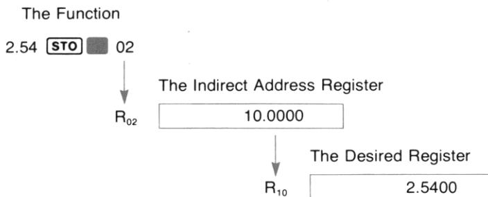
To recall numbers that are stored in any primary storage registers (R<sub>00</sub> through R<sub>99</sub>), you can simply press **RCL** and the number keys of the register address. You can also recall numbers from primary storage registers using indirect addressing, just like you did when you stored the number in the above example. Numbers in the extended storage registers (R<sub>(100)</sub> through R<sub>(318)</sub>) must be stored and recalled using indirect addressing.
