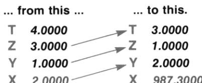
Then, when you press **ENTER**, the number is pushed into the Y-register. The contents of the stack are then changed...
