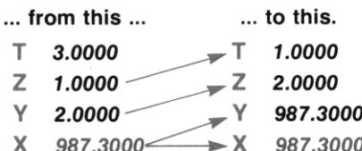
The value in the X-register is duplicated and *pushed* into the Y-register. The numbers in Y and Z are pushed up to Z and T, respectively, and the number in T is lost off the top of the stack.
