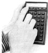
2. Turn the calculator over in your hand and push up on the lip on the battery holder as shown in the photograph.
