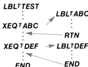
These subroutines have ALPHA labels grouped together, only the final one must be terminated with **END**.
