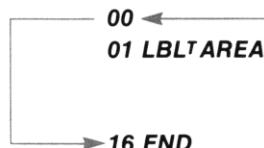
Pressing **BST** when the calculator is positioned at the top of the program moves the calculator to the end of this program.
