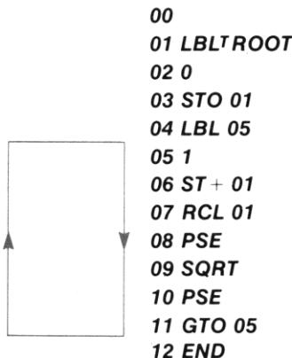
Looping techniques like the one illustrated here are common and extraordinarily useful in programming. By using loops, you take advantage of one of the most powerful features of the calculator—the ability to update data and perform calculations automatically, quickly, and, if you so desire, endlessly.
