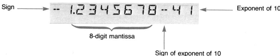
Scientific notation is selected by pressing **SCI** followed by a digit key to specify the number of decimal places to which the number is rounded. For example, place the speed of light (299,792,500 m/s) in the display and set the calculator to scientific notation.
