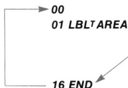
Pressing **SST** when the calculator is positioned here, moves the calculator back to the beginning of this program.
