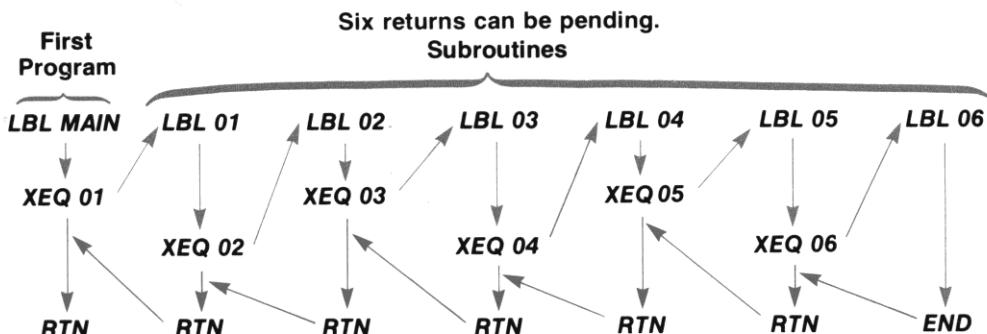
The calculator can return back to the first program from subroutines that are six deep, as shown. However, if you call up subroutines that are more than six deep, the calculator will return only six subroutines deep. For example, if you call up seven subroutines deep, when the seventh subroutine is completed, execution will transfer back only six subroutines, back to the second subroutine executed.
