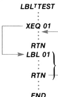
This subroutine has a numeric label and is terminated with **RTN**.
