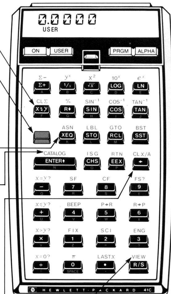
Views the contents of any register without disturbing the stack. To clear viewed data and return to the contents of the X-register, press ■.
