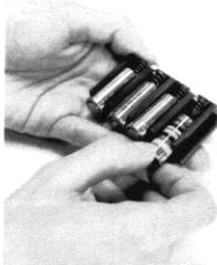
4. Look at the polarity marks on the end of the battery holder. It shows how the batteries should be inserted into the battery holder. Insert the new batteries, and *carefully note the position of each battery*. If any of the batteries are inserted wrong, the calculator will not turn on.
