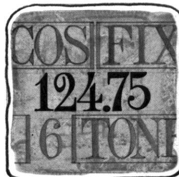
When a program line contains an instruction whose name is too long to display all at one time, the HP-41C “scrolls” the information through the display. Section 8 shows how **SST** and **BST** can be used to view these program lines.
