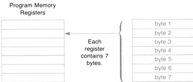
Most operations on the HP-41C require only one byte of program memory for storage as a line in a program, but some require two or even more bytes. For your reference, the number of bytes required for storing each programmable HP-41C function is listed in the table beginning below. The operations are listed in alphabetical order of their name.
