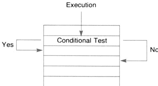
The line immediately following the conditional test can contain any instruction. The most commonly used instruction will be a **GTO** instruction. This will branch program execution to another section of program memory if the conditional test is true. For example:
