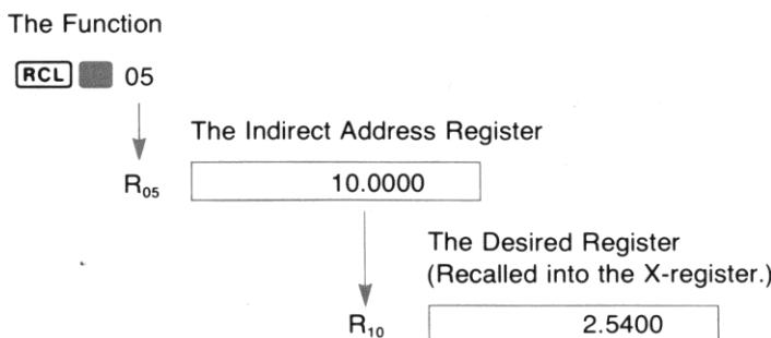
Storage register arithmetic is performed upon the contents of the indirectly addressed register by using **STO** **+** **nn**, **STO** **-** **nn**, **STO** **X** **nn**, and **STO** **÷** **nn**. If you do not remember how storage register arithmetic works, turn to page 74 to refresh your memory.
