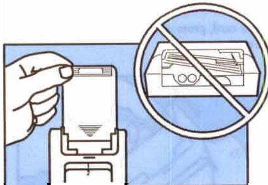
6. Slide the card firmly into the port until it stops. When you first feel resistance, the card has about  $1/4$  " to go to be fully seated.
