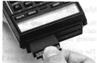
The information in an extended memory module is lost when the module is removed from the computer. **You can lose all data in two extended memory modules even if you remove only one of the two modules.** To avoid this, observe the following rules when choosing which of two modules to remove.
