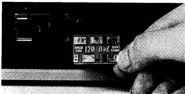
b. Position the line voltage selector such that the number indicating the required voltage setting is on the left.
