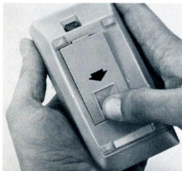
1. Turn the Power Switch to OFF and disconnect the battery charger from the calculator.
