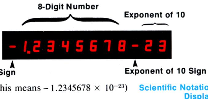
Scientific notation display is useful when you are working with large or very small numbers and allows all answers to be displayed with a specific number of digits after the decimal point. It is selected by pressing **DSP** followed by the appropriate number key to specify the number of decimal places to which the number is seen rounded. Again, the display is left-justified and includes trailing zeros within the selected setting. For example:
