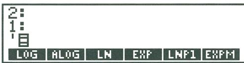
c. Press **EXP** **-** **N** **X** **LNP1** **I** **÷** **1** **0** **0** **ENTER** to put the expression on the stack. This expression takes advantage of the greater accuracy of LNP1 to calculate  $\ln(1 + i/100)$ .
