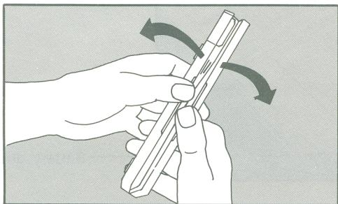
To close the calculator, fold the two sides together and press until you hear a click.
