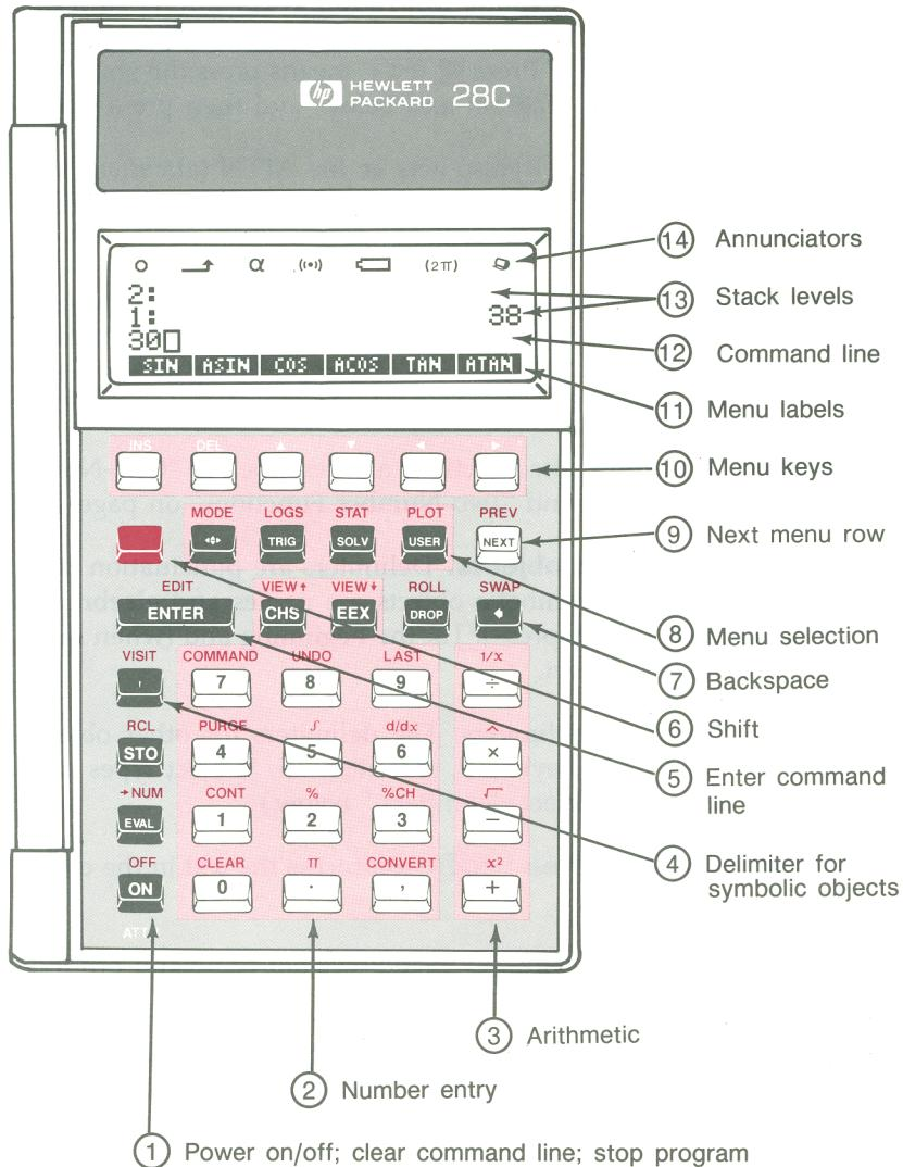
**1. Power on/off, clear command line, stop program.** To turn on the calculator, press **ON**; to turn it off, press **OFF**. (OFF is printed on the keyboard above **ON**. “Press **OFF**” means press the shift key **■**, which is item 6 in the diagram and below, and then press **ON**.)
