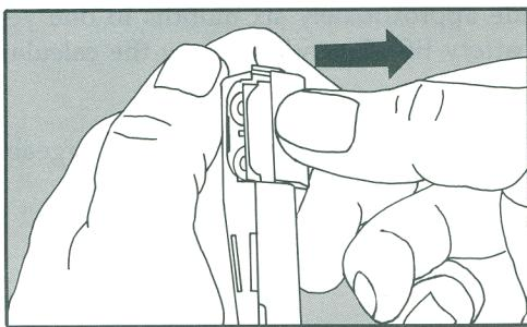
4. Tip the calculator to remove the old batteries.
