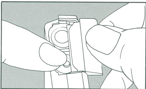
7. Slide the contact plate into the grooves. If necessary, use your finger to push the single battery into the compartment so that the door can slide over it. Slide the door until it latches into place.
