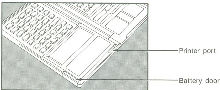
The HP-28C is powered by three N-cell alkaline batteries. Batteries are included with the calculator. If the batteries are not already installed, follow the instructions that start on page 213.
