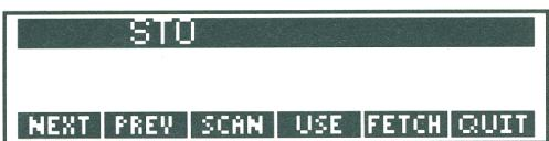
5. Press **USE** to show the usage for **STO**. The **USAGE** display shows that **STO** takes any object in level 2 and a name in level 1.
