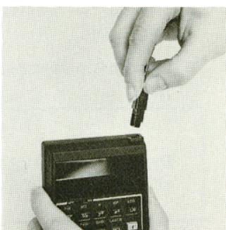
2. Press down on the battery door where indicated until the door release snaps open. Slide the door open.
