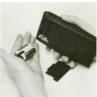
4. Place the new battery pack into the calculator. Your calculator will only turn on if the battery pack is inserted correctly.
