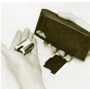
4. Place the new battery pack into the calculator. Your calculator will turn on only if the battery pack is inserted correctly.
