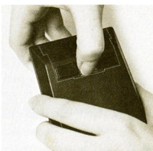
3. When door is removed, turn calculator over and gently shake, allowing the battery pack to fall into the palm of your hand.
