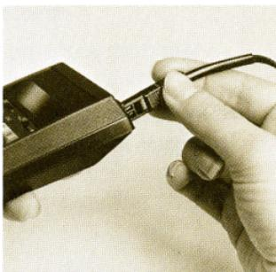
2. Press down on the short ridges of the battery door, close to the edge, until the door release snaps open. Slide the door open.
