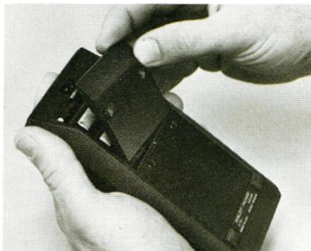
6. Insert the bottom of the battery door behind the retaining groove and close the door.
