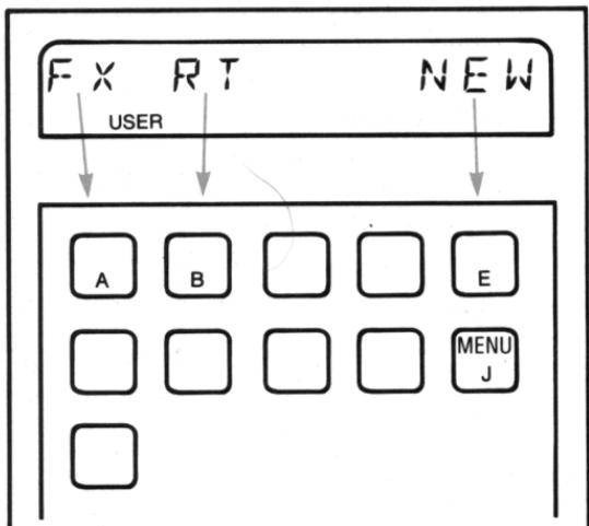
The **FX** menu label shows you that when you run PLY, the top left key on the calculator, **A**, is redefined to evaluate the polynomial  $f(x)$  at  $x$ . **B** (identified by the label **RT**) is redefined to compute the root, and **E** (identified by the label **NEW**) initializes the program to accept a new polynomial.
