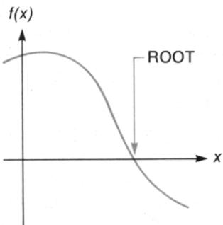
Executing the SOLVE program (**SOLVE**) employs an advanced numerical technique to find the real roots of a wide range of equations. You supply the equation for the function (in a program) and two initial estimates, and SOLVE does the rest.
