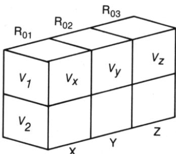
The vector stack is two vector-levels high, so it accommodates two vectors. Note, however, that each level contains *three* components: the  $x$ -,  $y$ -, and  $z$ -components for each vector.
