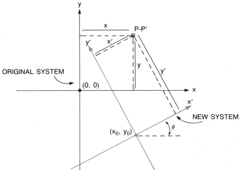
After specifying the new origin  $(x, y, z)$ , you specify the rotation angle. For a three-dimensional system with a non-zero angle of rotation, you also specify its *rotation vector*  $(a, b, c)$ . The rotation vector defines the axis about which the rotation is to be done; it can have any non-zero magnitude.
