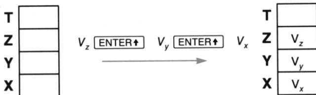
How do the two stacks relate to each other? Basically, the “*bottom*” level of the vector stack ( $V_2$ ) is stored in registers X, Y, and Z of the stack, while the “*upper*” level of the vector stack ( $V_1$ ) is stored in data storage registers  $R_{01}$ ,  $R_{02}$ , and  $R_{03}$ . You can imagine the registers shared in a three-dimensional stack like so:
