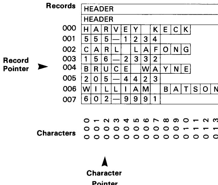
In the illustration, the record pointer is set to the fifth record and the character pointer is set to the third character. Taken together, the combination points to the **U** in **BRUCE WAYNE**. You can duplicate the ASCII file in the illustration by pressing the keys shown below. The **CRFLAS** and **APPREC** functions used will be explained later in this section (pages 24 and 29).
