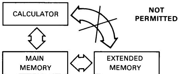
The registers in extended memory\* are organized in structures called "files." A program you create in calculator main memory can be transferred to extended memory as one type of file.
