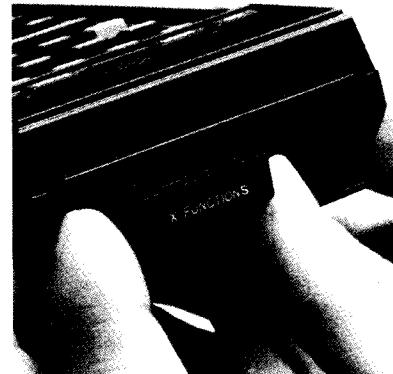
To remove a module, use your fingernail to gently extend the extractor handle. Then grasp the handle and pull out.
