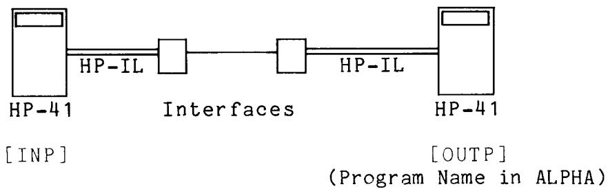
Each interface must be the primary device in its loop and must be properly initialized. The initialization and timing of the transfer depends on the interfaces. An example of program transfer using the HP 82168A Acoustic Coupler is provided on page 77 in appendix C.
