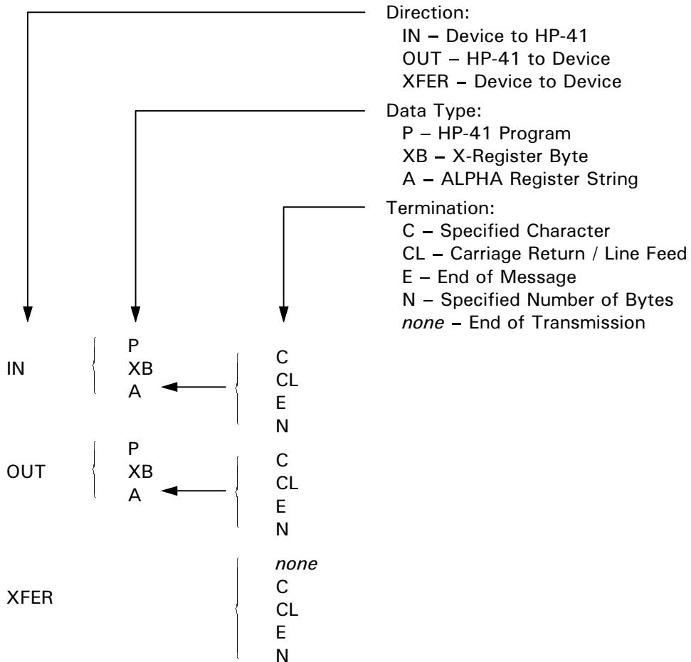
Thus, for example, you can translate **[INACL]** into IN + A + CL, to see that **[INACL]** reads bytes from the HP-IL into the ALPHA register and continues to add data bytes to the string in the ALPHA register until a carriage return / line feed is received.
