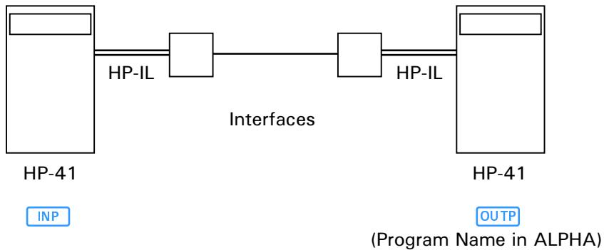
Each interface must be the primary device in its loop and must be properly initialized. The initialization and timing of the transfer depends on the interfaces. An example of program transfer using the HP 82168A Acoustic Coupler is provided on page 57 in Appendix C.
