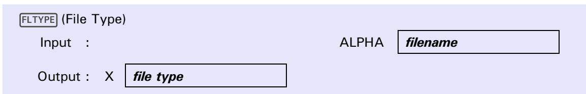
**FLTYPE** places into the X-register a two character Alpha string representing the type of the file named in the ALPHA register. The Alpha string corresponds to one of the file abbreviations used by the HP-IL module's **DIR** function:
