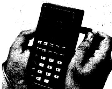
When the motor stops, remove the card from the left side of the calculator and insert it in the upper "window slot" on the right side of the calculator.
