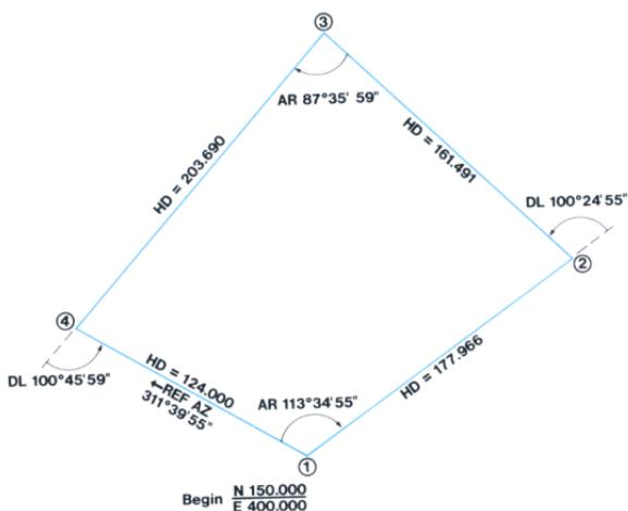
The field angles and distances for a traverse are shown on the figure. If the coordinates of the starting point are N 150, E 400, calculate the coordinates of the other points.
