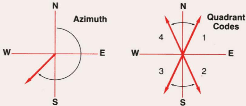
Thus azimuths are measured from the north meridian following North American surveying conventions. Bearings are measured from the meridian in the quadrant in which the line falls. Quadrant codes are shown in the above sketch.
