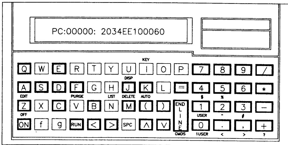
Figure 2. HP-71 Debugger Keyboard
