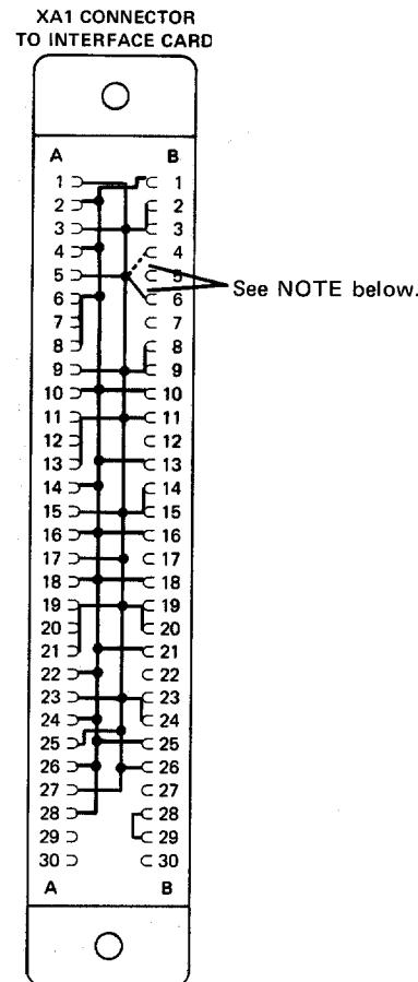
Figure 3-10. Test Connector Wiring Diagram
