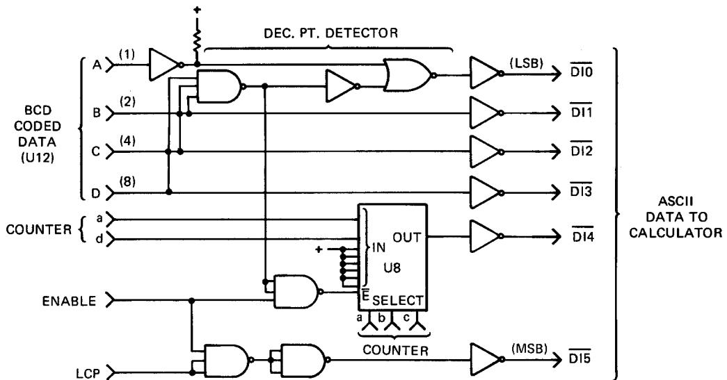
Figure 3-6. BCD to ASCII Converter
