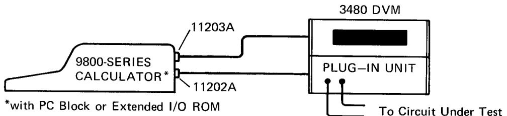
Figure 2-1. Typical Calculator/DVM System Configuration
