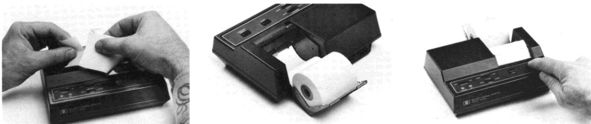
If the paper feeds properly but no printing appears, check that the paper is not installed backwards. The paper should feed from the bottom of the roll.
