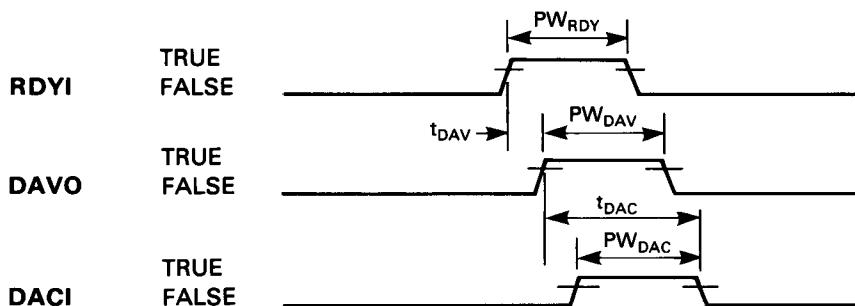
**Input (HP-IL  $\leftarrow$  GPIO) Timing:**
