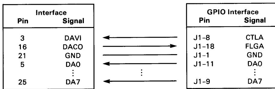
The next installation uses an 8-bit bidirectional data bus. The extra circuitry eliminates the need to modify the interface's control registers—the default values can be used. (The GPIO interface must have bit 0 of register 8 equal to 1—Output Enable A; other registers use their default values.)
