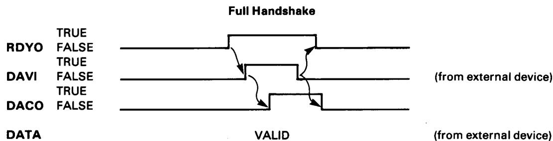
**Logic System.** The interface uses positive logic or negative logic for the data buses and for the handshake lines—each specified independently by control register R02-5,4.
