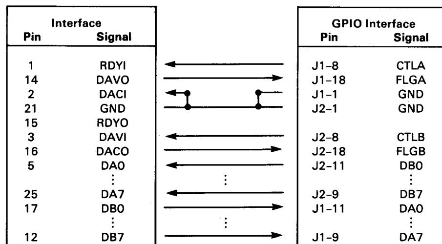
The last installation uses a 16-bit bidirectional data bus. Control register R02 must be set to 11001100 (value 204)—full handshake, positive data and handshake logic, 5- $\mu$ s time unit, 16-bit bidirectional data, disabled timeout; other control registers may be set to their default values. (The GPIO interface must have bits 1 and 0 of register 8 equal to 1—Output Enable B and Output Enable A; other registers use their default values.)
