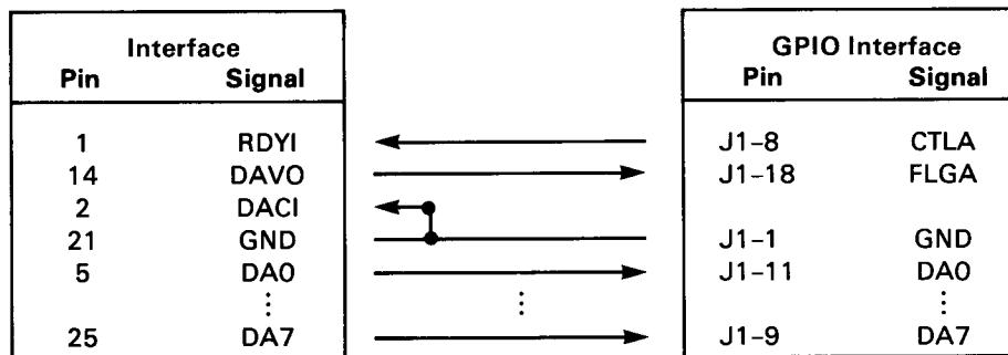
The second installation provides one-way communication from the GPIO interface to the interface. The interface uses the default values for its control registers. (The GPIO interface must have bits 4 and 0 of register 3 equal to 1—FLGA and CTLA negative-true—and bit 0 of register 8 equal to 1—Output Enable A; other registers use their default values.)
