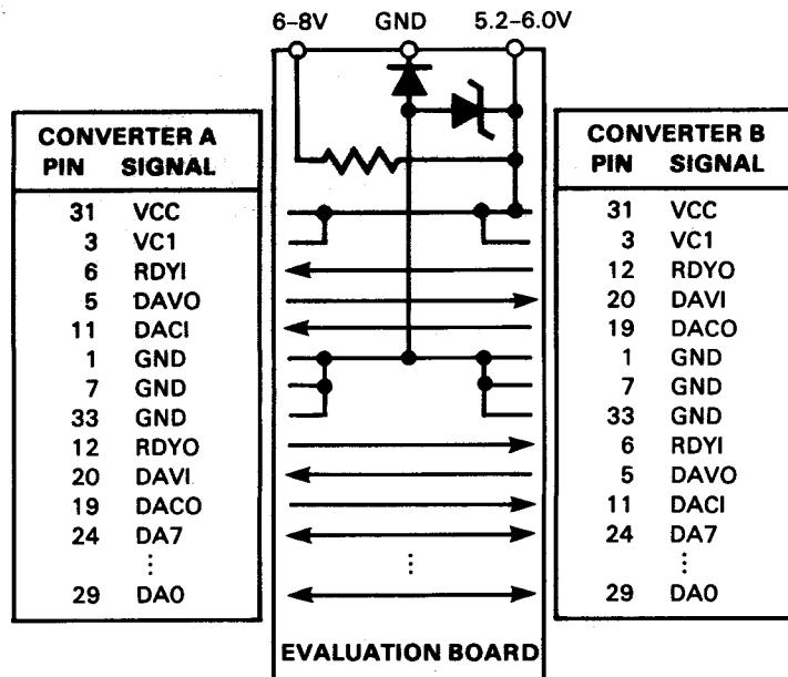
This connection can also be used to check the operation of two converters. You can join the interconnected converters in the same HP-IL system, then send data to one converter and retrieve it from the other. (Refer to appendix A.)
