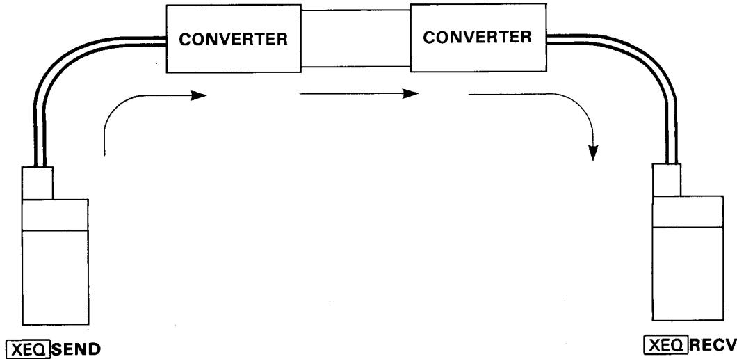
The following program is stored in each calculator. Execute RECV on the calcualtor that is to receive ALPHA data, and execute SEND on the calculator that is to send ALPHA data. Then enter a message at the sender followed by **R/S**.
