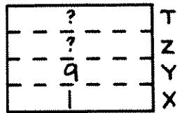
Line 009 asks the True-or False question: "Is the number in the X-register less than or equal to the number in the Y-register?" Since it is, the program continues with GT0 04. On the second time through the loop, 1 will be added to the X-register, and at line 008 (PSE) the stack will look like this:
