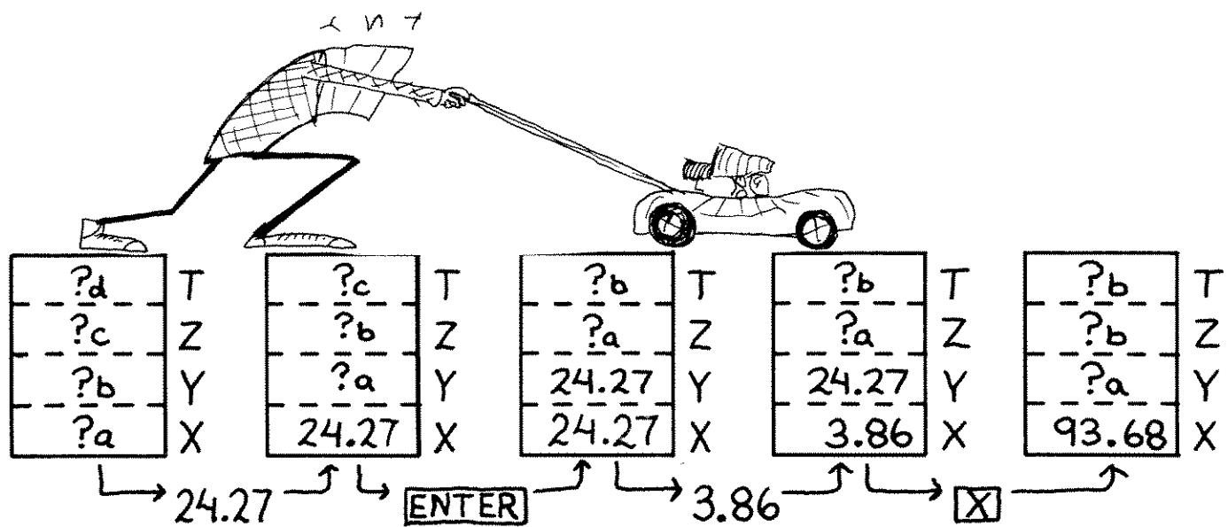
The above "stack-diagram" is a handy visual tool to demonstrate what's happening in the stack. The ?'s mean, "some number is there, but no one cares what it is." This is to remind you that there can be other numbers in the stack in addition to the ones you're working with, but they will never interfere. This means you don't have to clear all the stack registers everytime you start a new problem! And that saves both time and sore fingertips.
