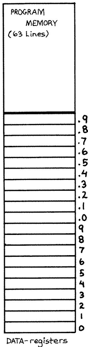
Each DATA-register can be converted into 7 lines of program memory.
