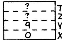
Line 005 begins the counting loop (LBL 4). On the first time through this loop, lines 006 and 007 add 1 to the X-register, and line 008 momentarily displays the X-register. Then the stack looks like this:
