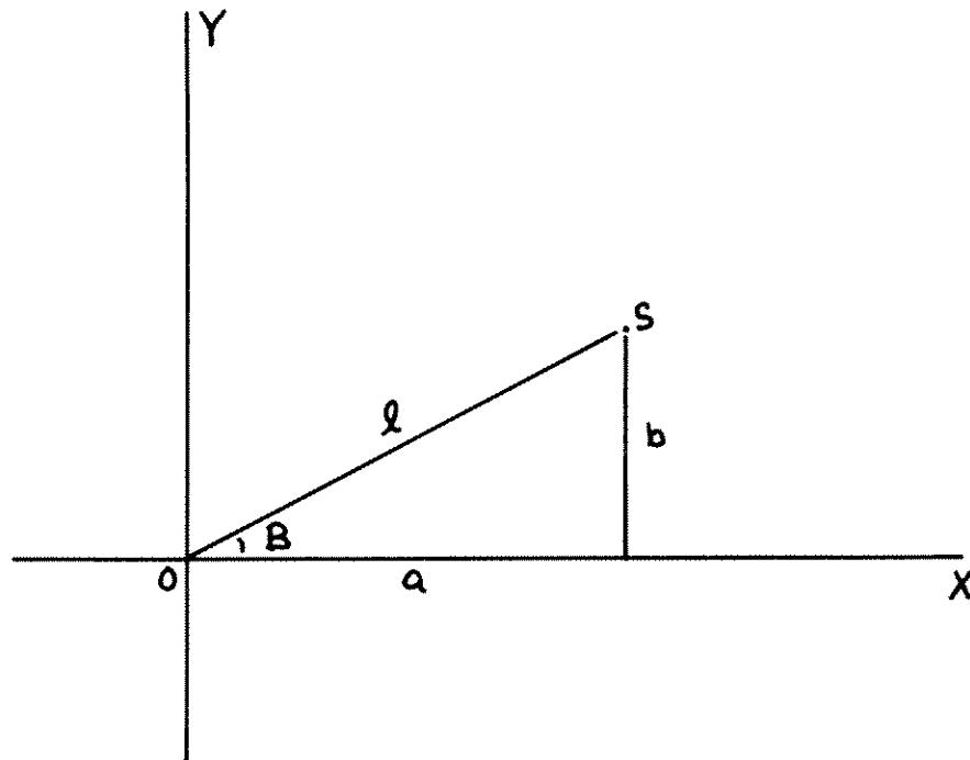
The names of these functions ( $\text{E}R$  and  $\text{EP}$ ) come from the fact that there are two ways of describing the location of point S.
