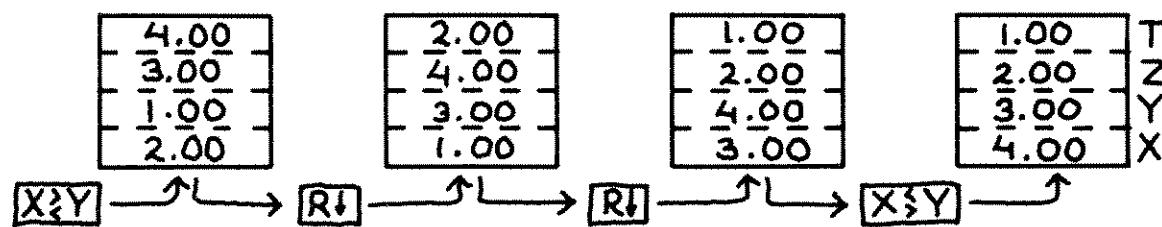
As you can see, the **R↓** (Roll Down) function rolls all the values in the stack down one register, and the value in the X-register is sent up to the T-register. The other function, **R↑** (Roll Up), does just the opposite. You can see where these names "Roll Down" and "Roll Up" come from.
