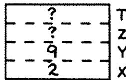
The program will continue to add one to the X-register, displaying the result, and testing the X-value against the Y-value until it reaches the tenth time through the loop. When it passes LBL 4 for the tenth time, the stack looks like this:
