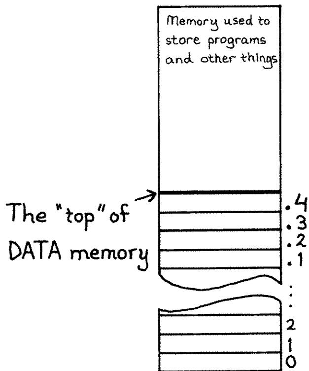
Now, try to store a number in register .9. Press 3.1416 **STO** .9. The calculator displays ERROR 3, and you blush--slightly. That means data register .9 (register 19) does not exist. The highest numbered data register is 14 (.4). Again, clear the ERROR message by pressing any key. Now try **STO** .4. It works. But try **STO** .5. You get ERROR 3, and more blushing. It's obvious where the boundary is, right?
