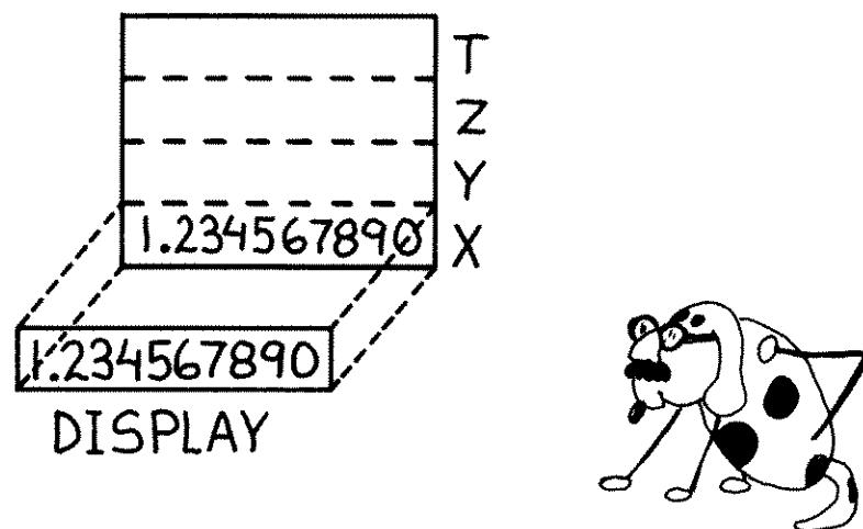
As you already know, the display is like a window over the X-register. And as you may have noticed, whenever you key in a number, this window slides open so you can see exactly what you're keying into the X-register.
