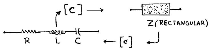
These are the only functions on the Equations Menu that don't try to interpret the format of the complex numbers you load into the stack (you load two complex numbers—four values). It takes you at your word: These are impedances either in Physical (R + L or C) or in Rectangular (R + X) form. It converts the (reactive portions of) the impedances back and forth:
