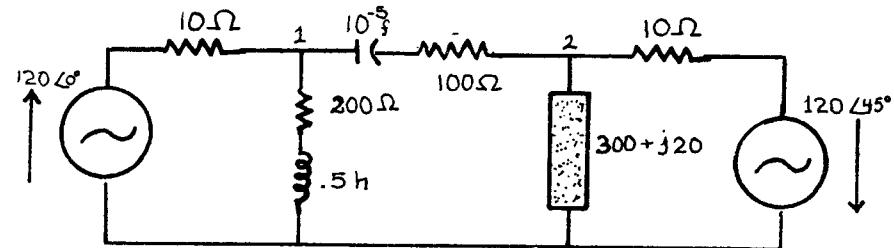
So if you have a circuit such as the one above, and you want to find the input impedance at nodes 1 and 2, do the following:
