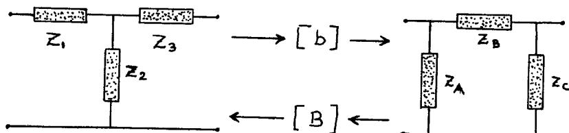
These are common calculations, often necessary to set up simpler circuit configurations. You load three impedances into the Complex Storage Registers A, B, and C, (because three complex numbers won't fit in the stack). Then select [b] to convert a Y configuration to a Delta, or [B] to convert a Delta to a Y.
