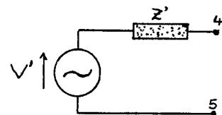
You can make this substitution PROVIDED that the  $V'$  is equal to the open circuit voltage difference across these same two nodes in the original circuit, AND that the  $Z'$  is equal to the input impedance at those two nodes.
