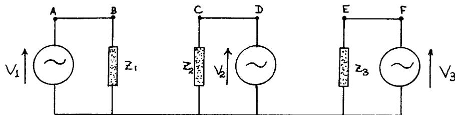
You will have to add negligible resistors between points A and B, C and D, and E and F, then use points B, C, and E as nodes.
