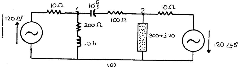
And suppose that, for more laughs, you wanted to calculate the voltages at node 1 and node 2, and the currents through the  $(300 + j20)$  impedance and the .5-henry inductor.
