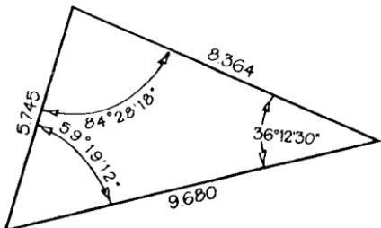
The notations for angles and sides is familiar to HP users, but is not the standard, or *textbook* notation which you have learned in trigonometry (side **a** opposite angle A, side **b** opposite angle B, and side **c** opposite angle C). The sides and angles are numbered, in order, going around the triangle.
