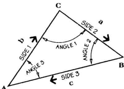
The example triangle (top) shows this style of labeling, compared to the standard notation for sides and angles. **Side 1** may be assigned to any side that is convenient to use, depending upon the available information about the triangle. It should be located at a side where the known information then falls into position for solution by one of the routines.
