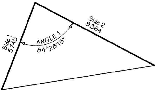
**TWO SIDES AND THE INCLUDED ANGLE KNOWN** is resolved by finding the third side, and then solving the triangle as shown on the previous page. The third side is found through the use of the equation
