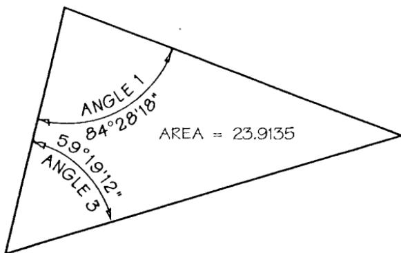
**AREA AND TWO ANGLES KNOWN** is first solved for the included side, and then solved as Angle, Side, Angle. The first angle input is treated as Angle 3, the second as Angle 1. The equation used for finding Side 1 is
