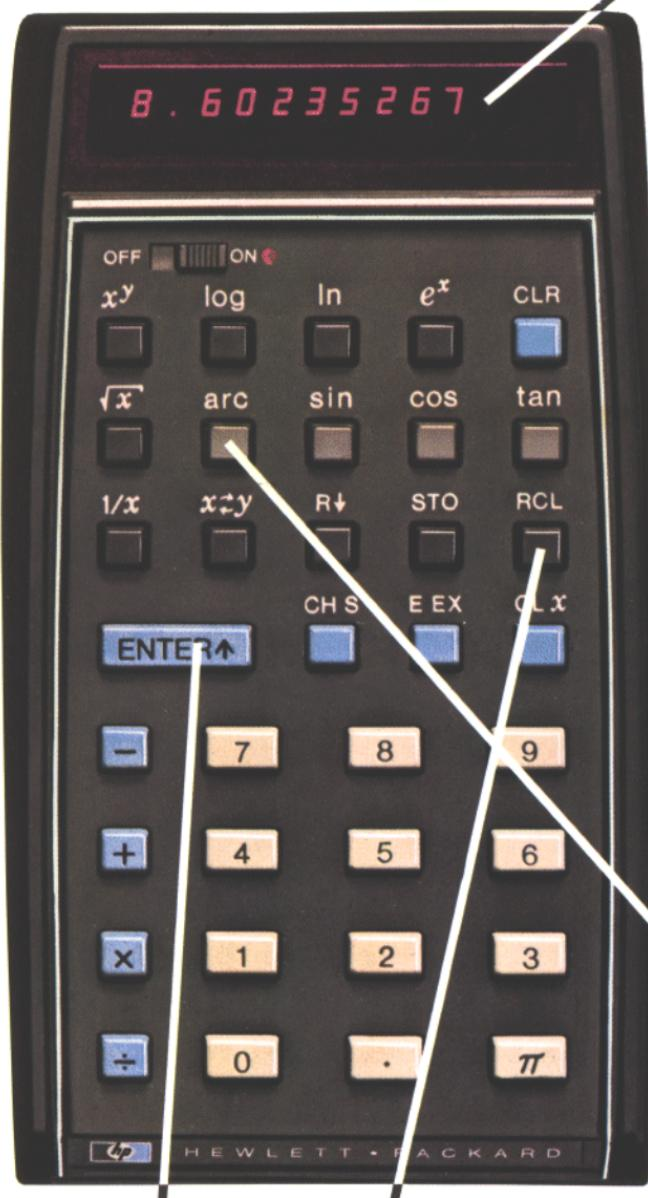
Provides "stack" of four registers plus one storage memory which can hold intermediate solutions to a problem and bring them back at appropriate time. Allows you to display for review.
