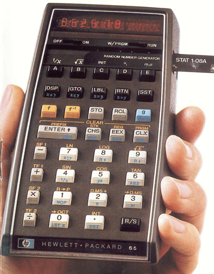
The HP-65's three prefix keys in row 3 enable each of the suffix keys to perform multiple calculating functions
