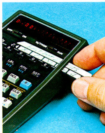
Label the program card and insert it in the slot above the User Definable Keys to identify them.
