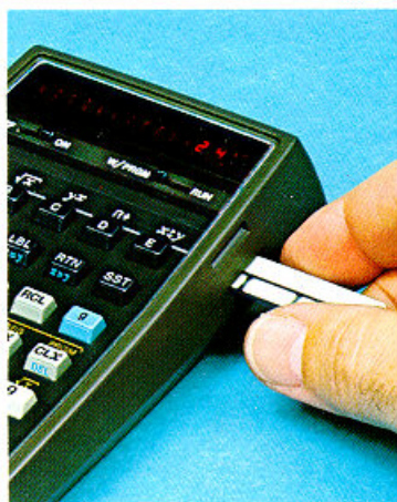
The resulting program is stored in the program memory as long as the HP-65 is left on. It can be permanently recorded by running a program card through the card reader.
