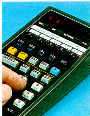
With the HP-65 set in the "RUN PROGRAM" mode, key in the known data for the specific problem you want to solve and run the program.
