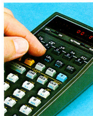
Then, with the HP-65 set in the "WRITE PROGRAM" mode, press the keys in the proper sequence.
