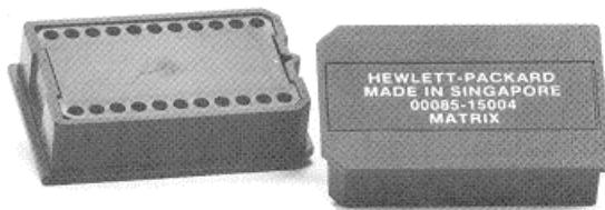
The Matrix ROM provides a powerful set of statements and functions for working with arrays—both matrices (two-dimensional arrays) and vectors (one-dimensional arrays). These capabilities enable array calculations to be performed with more convenience, speed, and accuracy than if they were done using an HP-85 alone.
