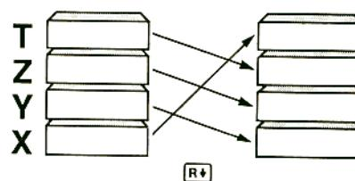
This feature provides for review of all current stack register contents. When used with  $X \Leftrightarrow Y$ , it provides a means for rearranging the four arguments in any fashion.
