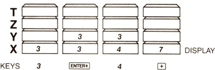
Notice that just before the + key is pressed, the two numbers are logically arranged in the stack the same way as they would be if the problem were being worked by hand:
