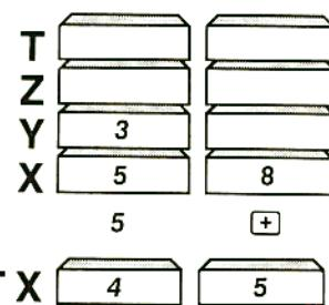
In a similar manner, if the wrong function key was pressed, a user can recall LAST X, reverse the function, and then proceed with the correct operation.
