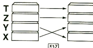
This capability is useful in divide and subtract operations, where the order of the X and Y contents is meaningful.
