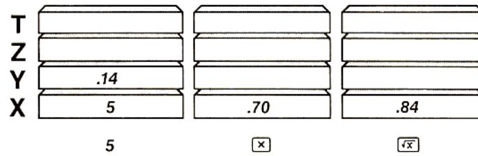
The HP RPN system enabled this calculation to be attacked and worked in the same order as if it were worked longhand with pencil and paper.
