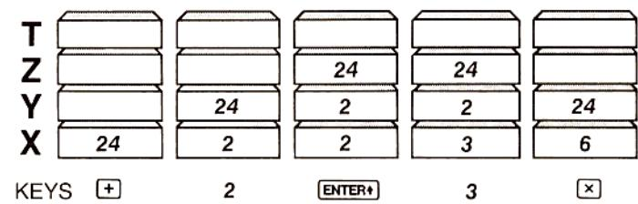
Again, the two intermediate results  $(12 \div 3) + (5 \times 4) = 24$  and  $(2 \times 3) = 6$  are positioned in the X and Y registers for the next step in the calculation:
