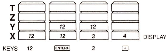
This is the first intermediate result,  $(12 \div 3) = 4$ . This intermediate result is automatically kept by the stack while the next intermediate result  $(5 \times 4)$ , is calculated.
