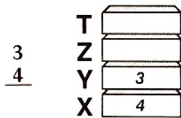
The effect of the ENTER key was to copy the number 3 from the X register into the Y register, leaving the X register ready to receive the second number. When the + key is pressed, the numbers in the X and Y registers are added together, and the result appears in the X register. Consider a more complex problem:
