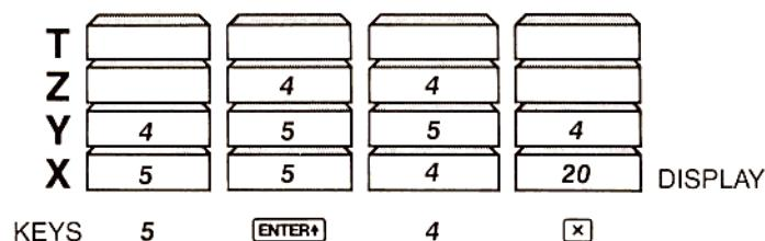
This is the second intermediate result,  $(5 \times 4) = 20$ . Above it, in the Y register, is the previous intermediate result,  $(12 \div 3) = 4$ . Both intermediate results are just in the correct positions, the X and Y registers, to be
