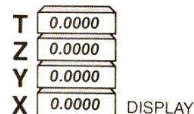
In the illustration there are the four registers, each one with a letter name that is used to refer to that particular register. Note also that the X register is the display register; that is, the number you see in the calculator's display is **always** the number in the X register.
