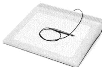
This device is a high-quality graphics tablet that can be used to create or locate graphical data or as a display for interactive graphics applications.
