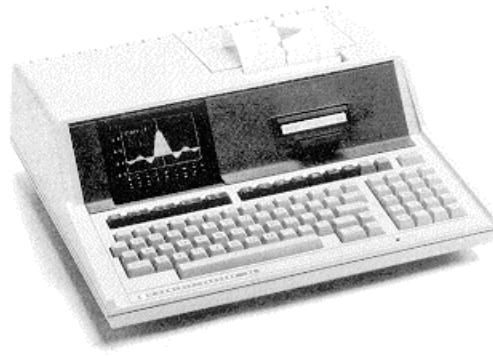
A powerful BASIC language computer complete with built-in keyboard, CRT display, printer, tape unit, and graphics system.
