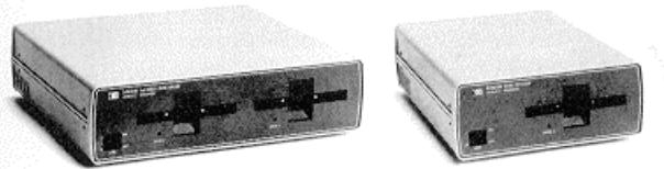
Each removable flexible disc supplies approximately 270K bytes (formatted) of on-line storage. You must start with a master drive. Each master can support one add-on drive for a maximum of 1,080K bytes using a HP 82901M Dual Master and a HP 82901S Dual Add-on Drive.
