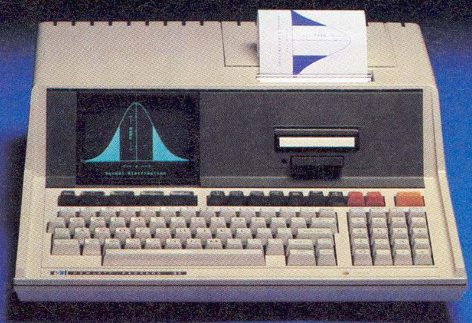
At the heart of the HP-87 is HP's enhanced BASIC language—a language that's simple to understand, yet powerful enough to handle difficult technical problems. HP BASIC on the HP-87 features string arrays, multi-character variables, line labels, multi-parameter functions, multiple binary programs, formatted program listings, and graphics, printer, and mass storage commands.
