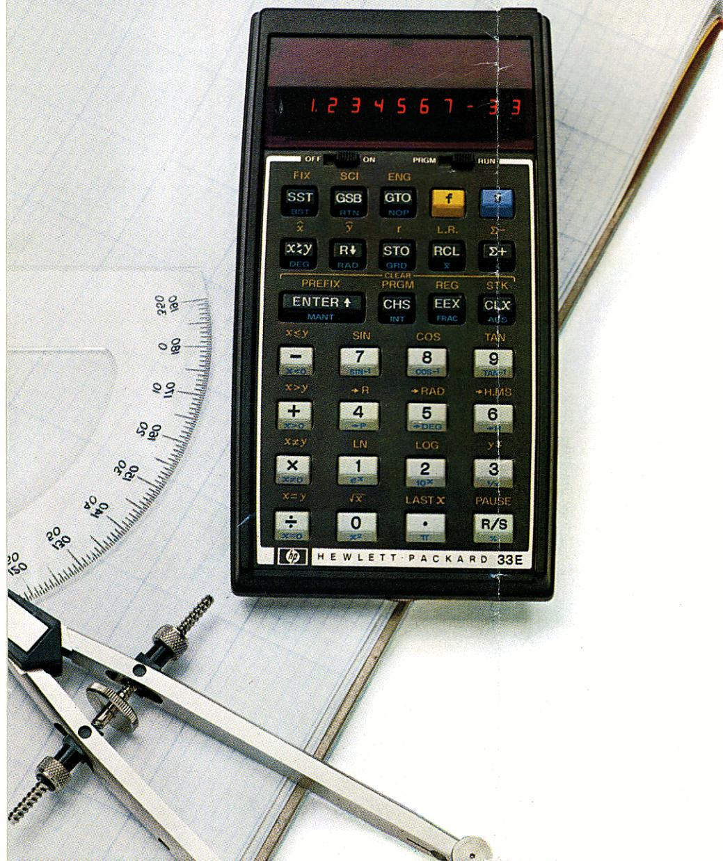
The HP-33 is an advanced scientific calculator that is also programmable! Like its famous predecessor the popular HP-25, the new HP-33 remembers a series of keystrokes as you press them, then executes the sequence later at your command. But the HP-33 has a combination of features we've never before offered on a key-stroke programmable calculator—including a new low price.
