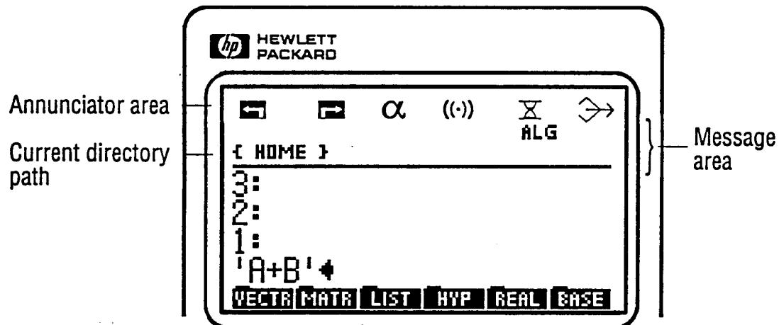
Figure 2 - Typical HP 48 Display showing HP 48 annunciators.
