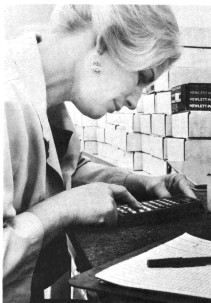
7. When the calculator passes all electronic tests, it is sent to the Quality Assurance Station. Here, the operator inspects the overall appearance of the calculator, and runs a final set of test calculations.
