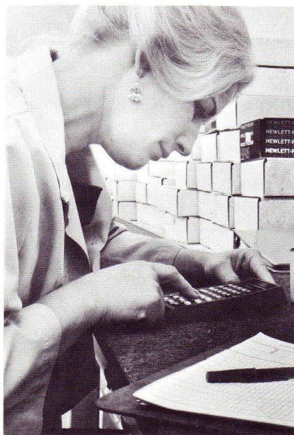
7. When the calculator passes all electronic tests, it is sent to the Quality Assurance Station. Here, the operator inspects the overall appearance of the calculator, and runs a final set of test calculations.
