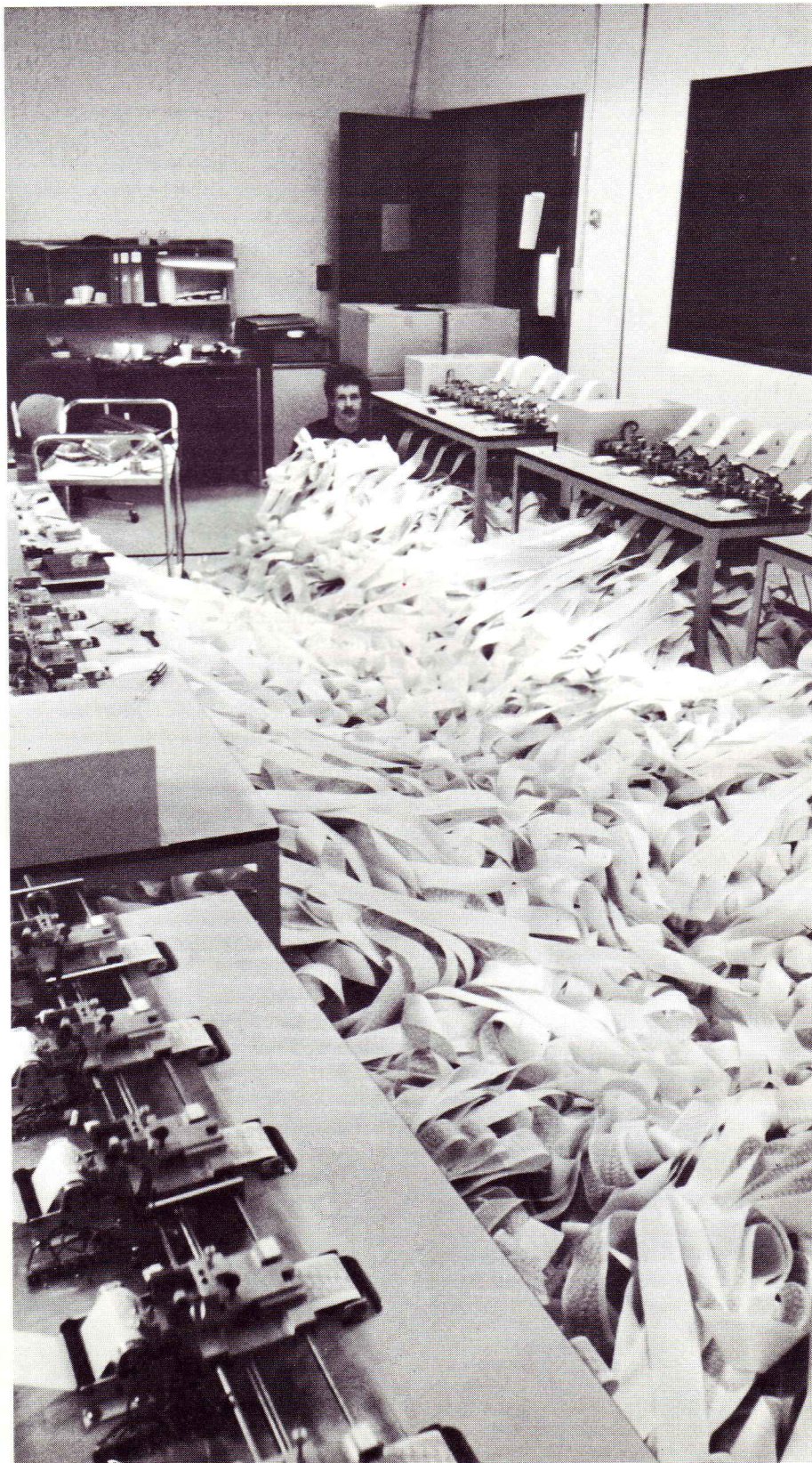
Before paper take-up rollers were installed, thermal paper filled the testing room over weekends.
