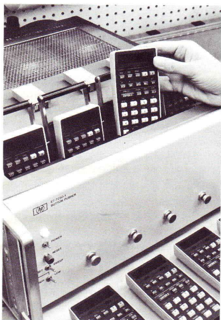
6. An electronic "button-pusher" runs the logic board through a sequence of calculations to make sure the keyboard works perfectly.
