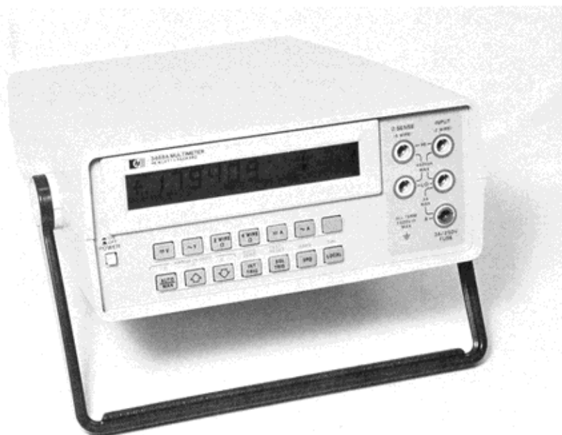
Fig. 1. The HP Model 3468A Multimeter is HP's first HP-IL instrument. It has an alphanumeric liquid-crystal display, measures ac and dc voltage and current, and determines resistance by both two-wire and four-wire methods.
