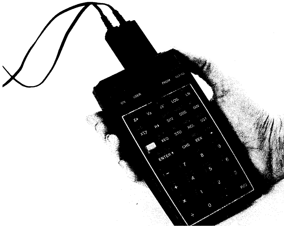
Fig. 5. When a user plugs the HP 82160A HP-IL Module into one of the four I/O ports in the HP-41CV Programmable Calculator, the calculator becomes a portable system controller, able to interface with a variety of peripherals. Through the HP-IL, the HP-41CV can control a graphics plotter (see last month's issue, page 16), display data on a video monitor, transmit data over telephone lines to a larger Series 80 Computer, and collect measurements in the field.
