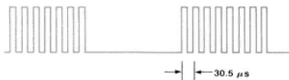
Fig. 2. Data is transmitted as a series of bursts of infrared light, each burst formed by six to eight pulses of energy at a pulse repetition rate of 32.768 kHz.
