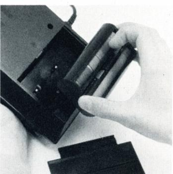
5. Insert the end of the battery door that is opposite the latches behind the retaining groove, and close the door.
