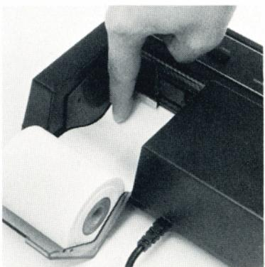
4. Press the paper advance key and hold it down until the paper passes the top of the plastic tear bar.
