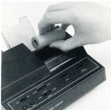
2. Before inserting the new roll of paper into the printer, discard the first two turns to ensure that no glue, tape or other foreign matter is on the paper. Make sure that the leading edge of the paper is straight, not crooked or jagged. A short, sharp crease on the leading edge may aid in the loading of the paper.
