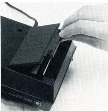
6. Secure the door by pressing it gently while sliding the two battery door latches outward.
