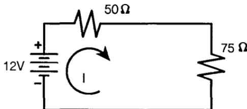
The total current  $I$  can be found easily since the  $50\Omega$  and  $75\Omega$  resistors are connected in series giving a total resistance of  $50 + 75 = 125\Omega$ . The total current  $I$  is then found using Ohm's Law of  $I = V/R$ .
