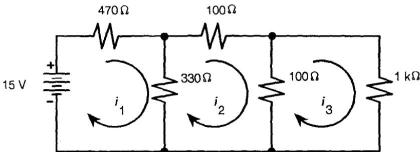
The following three equations are generated by summing the voltage drops around each loop.
