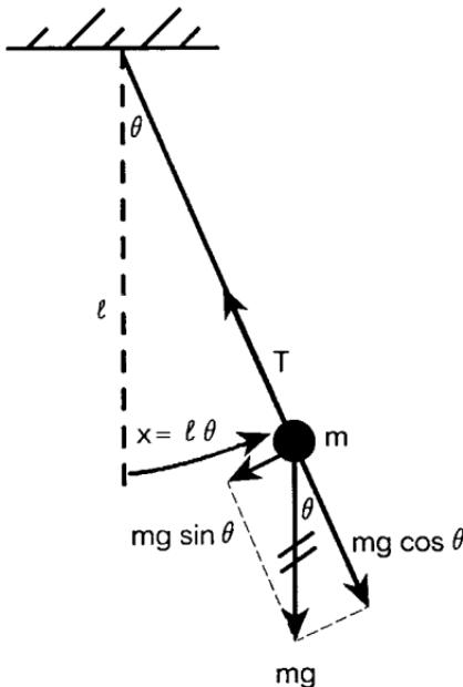
As shown in the figure, the restoring force in a simple pendulum is  $F = -mg \sin \theta$ , and the displacement is given by  $x = l\theta$ . For small angles  $\sin \theta \approx \theta$  and the restoring force becomes
