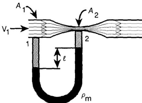
The U-shaped tube in the figure is called a manometer\* and is used to measure pressure differences. The manometer equation for pressure difference is
