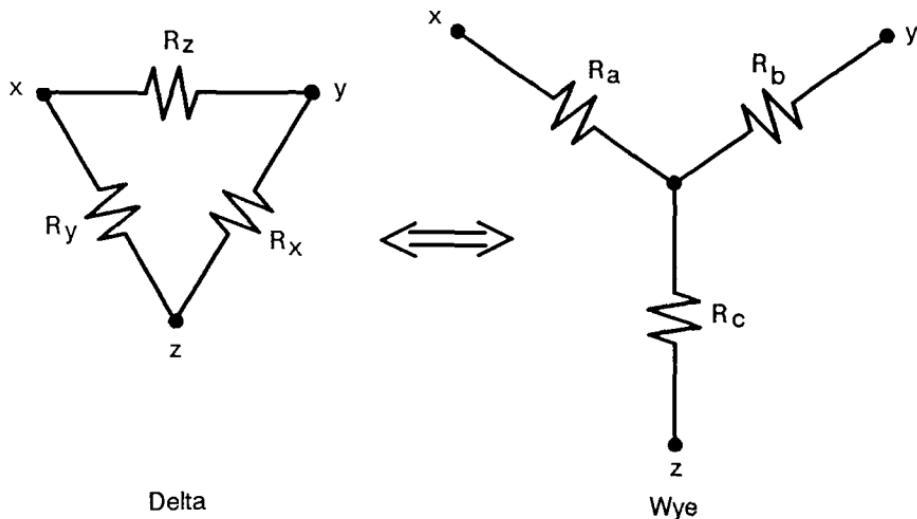
Circuit analysis is sometimes simplified by transforming a  $\Delta$  configuration to a Y configuration or vice-versa. The formulas below show how to do this.
