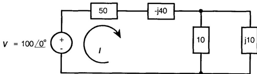
The impedances in parallel are converted to an equivalent impedance using a special case of the parallel impedance formula when there are only two impedances
