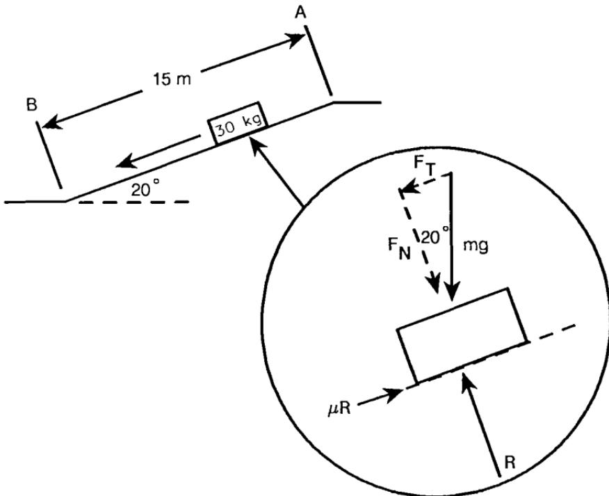
The free body diagram is shown enlarged in the figure. The normal force  $R$  is equal and opposite to  $F_N$ , the normal component of the crate's weight. From the figure, this is
