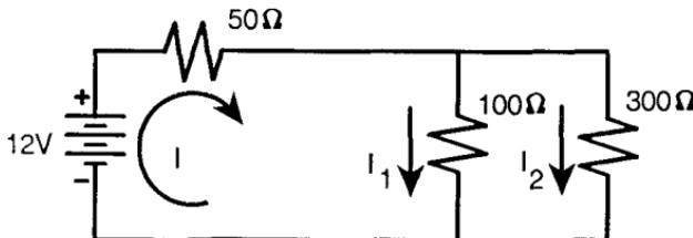
To solve this problem, first find the total current  $I$  by finding the equivalent resistance of the circuit. The  $100\Omega$  and  $300\Omega$  resistors are connected in parallel. The formula for parallel resistance becomes
