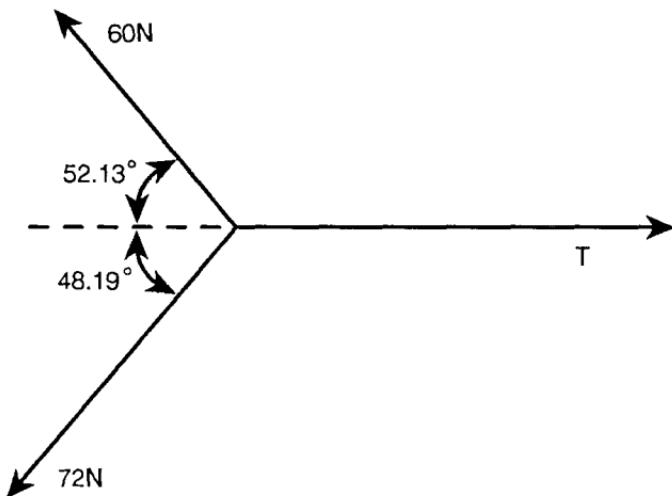
From the figure, it is clear that  $T$  must be such that the sum of forces in the x-direction is zero.  $T$  contributes no force in the y-direction since the sum of forces is already zero in that direction.
