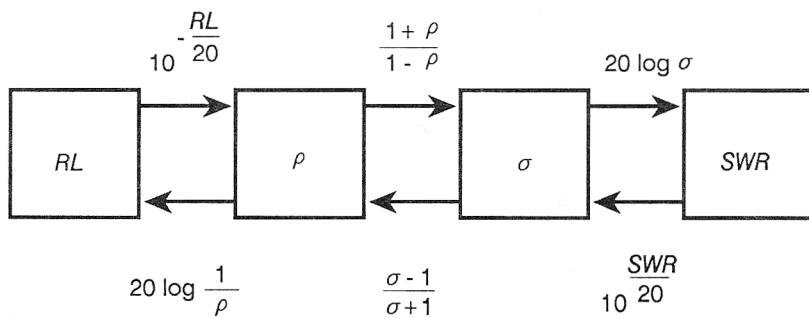
For a system having characteristic impedance  $Z_0$ , the impedance and reflection coefficient are related by
