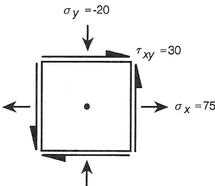
Find the principal stresses and their orientation, and the stresses on the face of the element oriented 45° counterclockwise from the  $x$ -axis.
