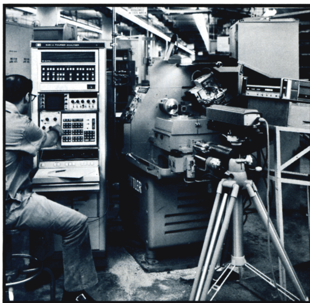
Fig. 2. New Model 5451A Fourier Analyzer, a minicomputer-based, keyboard controlled, dual-channel analyzer, can do spectrum analysis, correlation, coherence analysis and many other complex data manipulations. New capabilities are 80-dB dynamic range, relocatable software, buffered input, and a faster computer.
