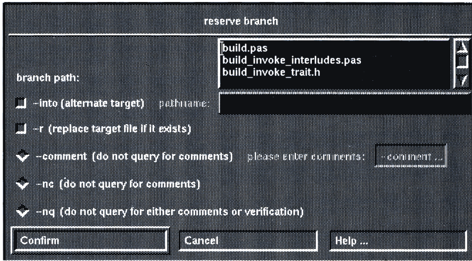
Fig. 9. A dialog box that provides multiple iteration. The box contains a scrollable window containing element names. Users can select one or more of these names and DSEE will issue a separate reserve branch command for each selected element name.
