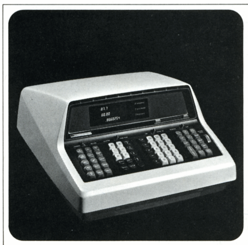
Fig. 1. (left) This new HP Model 9100A Calculator is self-contained and is capable of performing functions previously possible only with larger computers. Fig. 2. (right) Display in fixed point with the decimal wheel set at 5. The Y register has reverted to floating point because the number is too large to be properly displayed unless the digits called for by the DECIMAL DIGITS setting is reduced.
