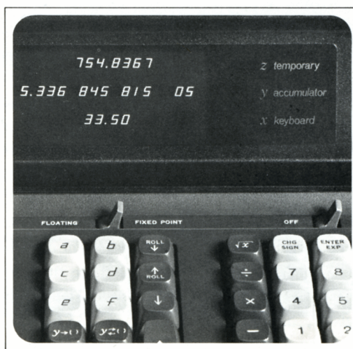
Fig. 1. (left) This new HP Model 9100A Calculator is self-contained and is capable of performing functions previously possible only with larger computers. Fig. 2. (right) Display in fixed point with the decimal wheel set at 5. The Y register has reverted to floating point because the number is too large to be properly displayed unless the digits called for by the DECIMAL DIGITS setting is reduced.
