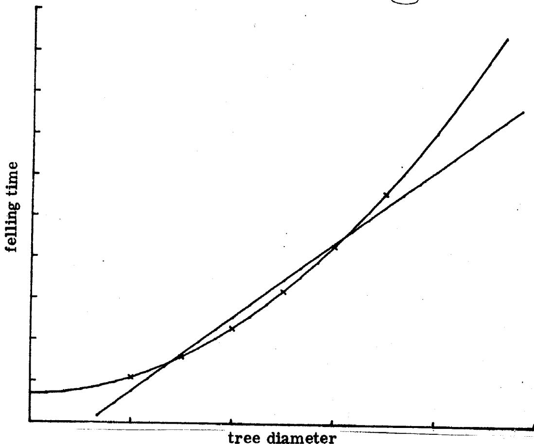
Notice the parabolic curve goes through all the data points, whereas the linear curve fit does not.
