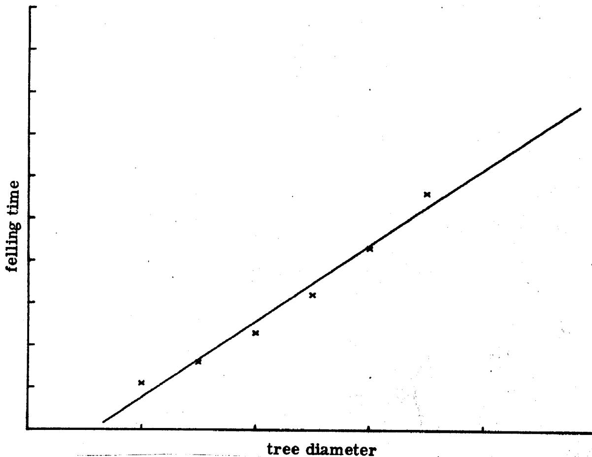
We readily notice that the felling time is not linear. This should not come as a surprise because tree area increases as the square of the tree diameter. Thus, a parabolic model would probably yield a better fit.
