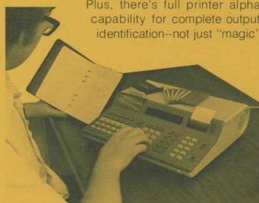
combinations of symbols to decipher. The keyboard has full trigonometric capability plus 15 special function keys. These special keys are used as program and routine loading keys. Pressing a single special key accesses and starts a program or routine. Each key is easily identified by a template which slips over the block of 15 keys.
