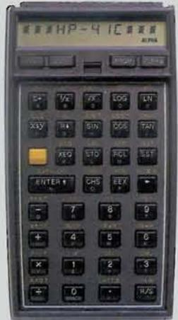
TWO HP-41C'S, CARRIED BY ASTRONAUT ROBERT CRIPPEN, ABOARD THE SPACE SHUTTLE COLUMBIA, contained critical programs. One to tell *Columbia* the next ground station to contact, when contact would be made and for how long. The other to calculate both the pre-entry center of gravity (balancing point) and the amount of fuel that must be burned to maintain the precise balancing point during descent.
