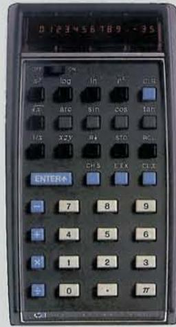
THE HP-35, THE WORLD'S FIRST HANDHELD SCIENTIFIC CALCULATOR orbited in space aboard three manned *Skylab* missions (1973-74). Solar research figured prominently among the wide assortment of experimental research conducted. Used as a backup to on-board computers, the HP-35 calculated predocking rocket burns necessary to align the Apollo Command Module with *Skylab*. In addition, the HP-35 helped *Skylab* crews aim their telescopes at stars in attempts to measure ultraviolet radiation.
